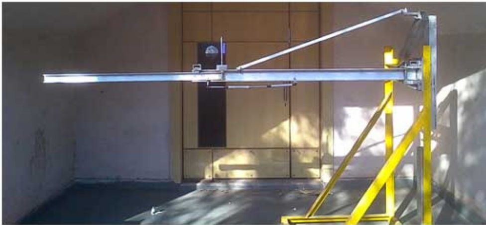
Illustration: Prototype of deployable boom assembly
